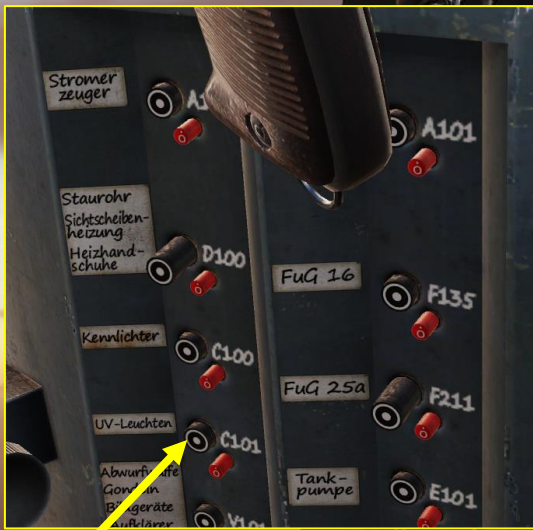
C101 Interior UV Lights Power Switch (UV Leuchten)
