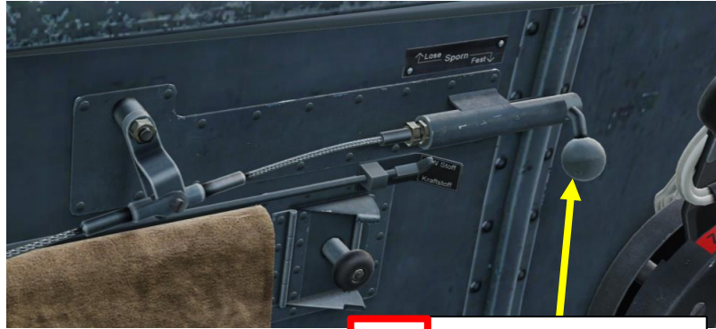
2 Tailwheel Locked ("L-shaped" position)
